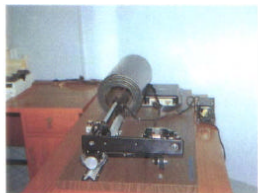
The spinner magnetometer (SSM-2) is used for measuring the remanent magnetisation rocks.
