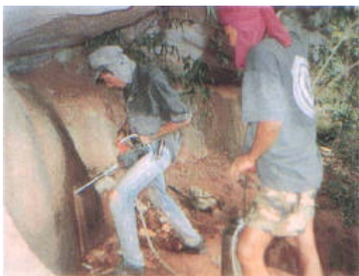
The palaeomagnetic cored specimens (25mm. In diameter) were collected by drilling with hand-drilling machine.
