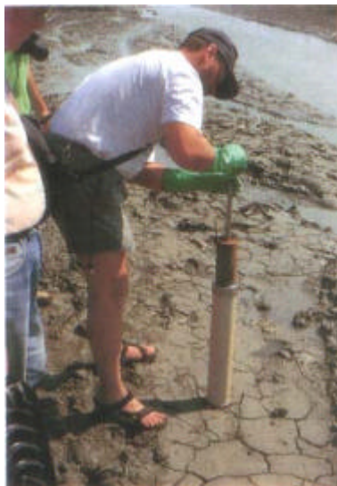
Showing the collection of coastal clay sample (undisturbed-sample) in order to be analysed by means of physics, chemistry and paleontology.
