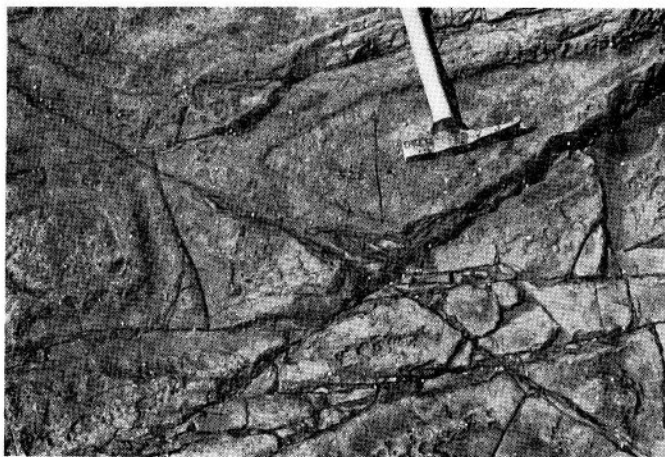
Fig. 8 B-la set ; running from left upper to right below. B-lb ; from right upper to left below. B-lc ; running horizontally.
