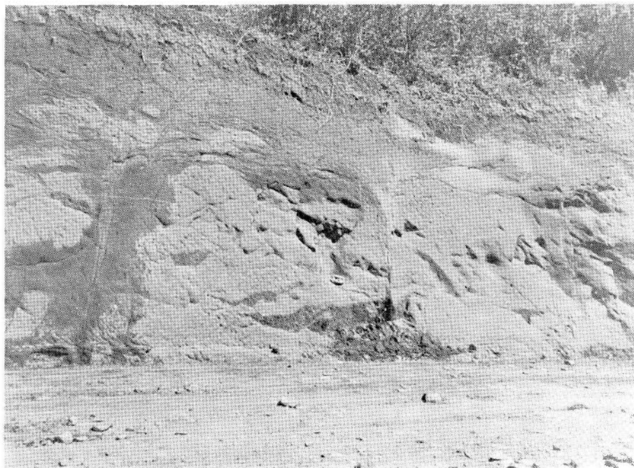
Photo 1. Joints in loose, coarse sandstone of Iwaki formation. The sandstone is found to form reservoir beds at most wells. Interval among joints is wider than any other rocks in this field. A cap in the middle is a scale indicator. View at the roadside in Idekura, Nakoso city.
