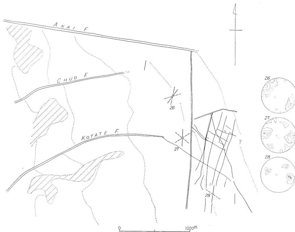
Fig. 12 Fractures map-6 Area (e) in the subsurface Iwaki formation, Taira area
