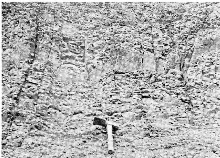
Photo 2. Joints in shale of Shirasaka formation. Numerous weathering joints are formed among larger, straight-lined systematic joints which have nearly vertical or steep dip. The weathering joints of this kind were excluded from measurements. Both views are found near Hattan, Nakoso city.
