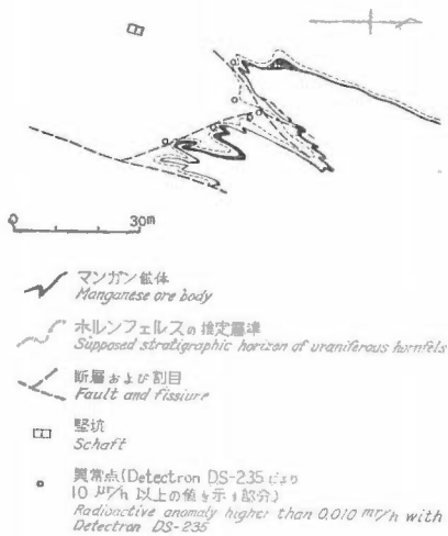
第6図 -90m坑の異常点分布 Distribution map of radioactive anomalies in -90m level, Nodatamagawa mine
