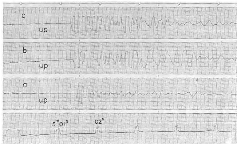
Fig. 5-37 Seismograms obtained (109) at D 11 , (110) at D 12 and (111) at D 13 from the shot A-V 2
