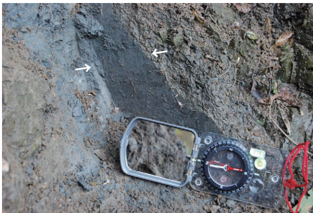
第3図 未固結粘土状の断層ガウジ. Fig.3 Fault gauge as unconsolidated clay.
