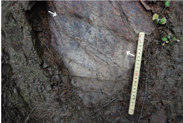
第2図 固結粘土状の断層ガウジ. Fig.2 Fault gauge as hard consolidated clay.
