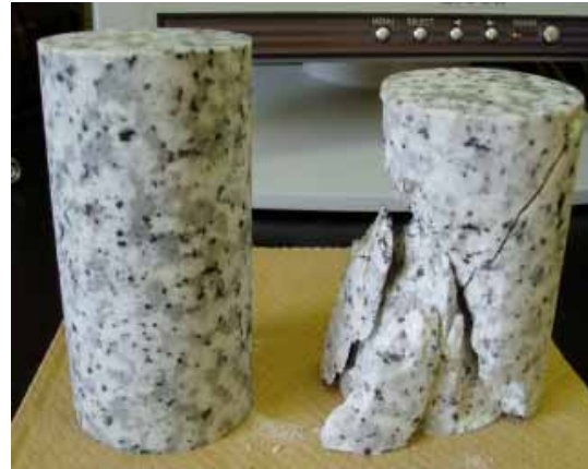
Inada Granite (Ibaragi, Japan) Size: 0.5-4.0mm Quartz 31%, Feldspar 63%, Biotite 4%
