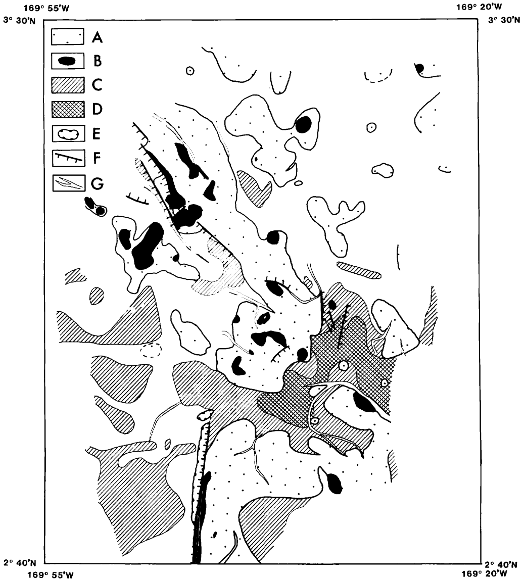
Fig. III-5 Surface acoustic character distribution map in the GH81-4 survey area. A: knoll or topographic high area. B: basement exposed area. C: thin and vague stratification distributed area. D: thick and clear stratification distributed area. E: depression area. F: steep scarp. G: channel.
