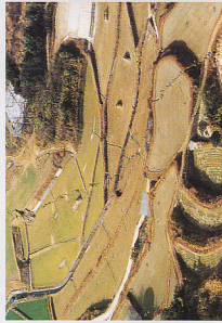
Earthquake surface fault along the Nojima fault (Awaji Island) (by Asia Air Survey)
