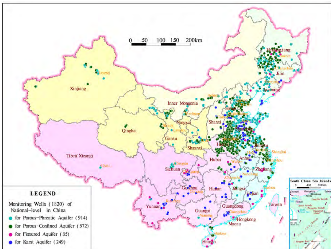
Fig. 2 Distribution of the National-level Monitoring Wells in China
