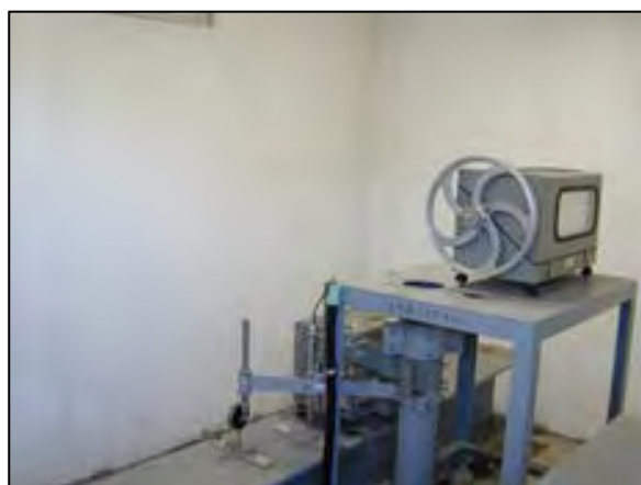
Photo 1 Observation well for monitoring of groundwater level and land subsidence in Japan (left), digital thermistor with 300m cables (right), respectively.
