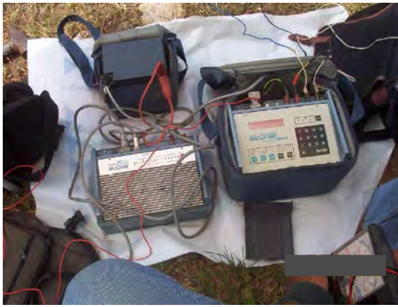
Photos 1 and 2 - The OYO McOHM Mark-2 Model 2115A resistivity instrument used during the geo-resistivity survey with MGB-ROITeam.
