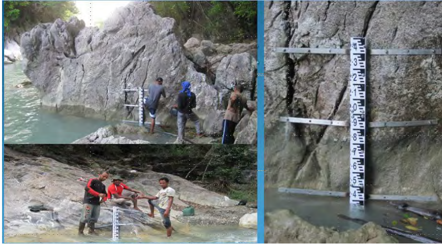
Figure 10. Meter installation or stream gauge in Balubo river-Maliana District. (source: DNCQA,
