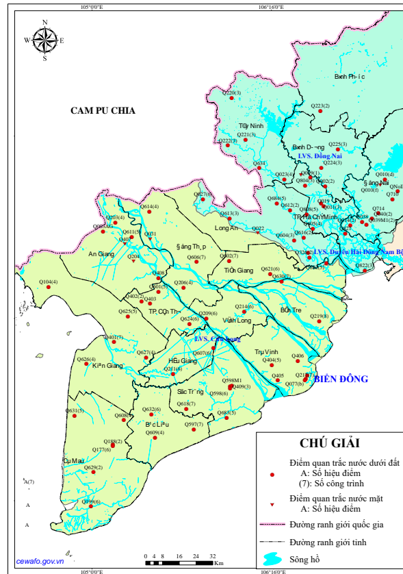
Fig. 3. Diagram of the groundwater resources monitoring network in the Mekong River Delta region
