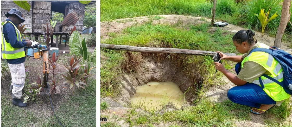
Fig. 2. Photographs showing usual site inspection of bores and shallow wells during groundwater investigations
