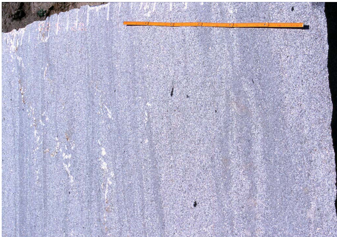
Fig. 13 Muscovite-biotite granite showing heterogenous mineral compositions, Nakane-Sekizai quarry, Aichi Pref. The yellow scale is 1 meter. The black patches are restitic biotite aggregates, which are dominant in salic layers.
