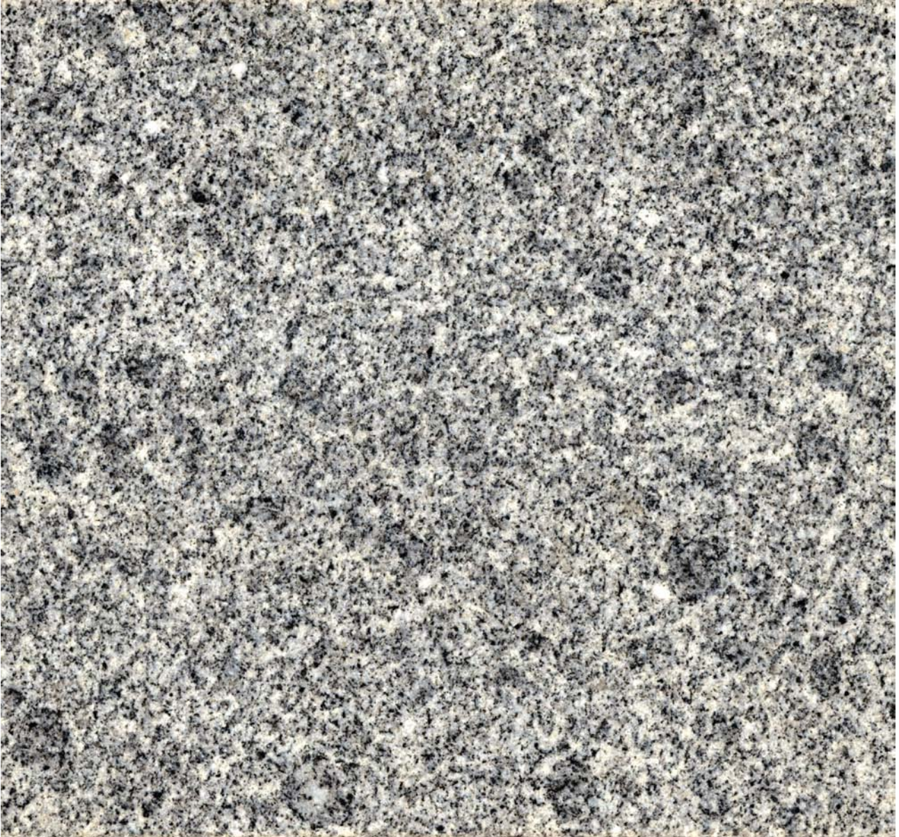
Fig. 2 Heterogeneous looking of Aji Granite, which is considered the best-grade tombstone in Japan. Tabuchi Quarry, Aji township, Kagawa Prefecture (x1).
