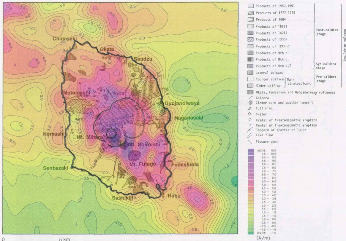
Fig. 7 Apparent magnetization intensity map of Izu-Oshima volcano, Japan, superimposed on a geologic map of the volcano before the 1986 eruption (Sakaguchi *et al.*, 1988). Contour interval is 0.5 A/m.
