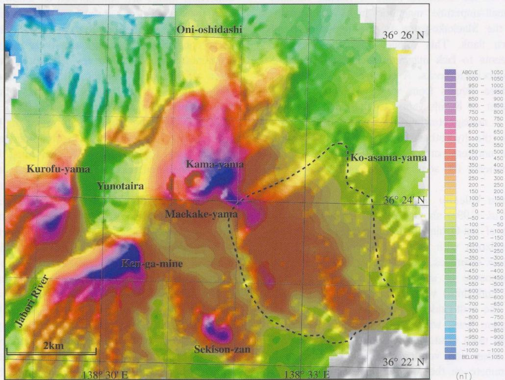
Fig. 6 Reduction to the pole anomaly map of Asama volcano with a topographic shading. The data was reduced onto the smoothed observed surface. Contour interval is 50 nT. The area bound of broken lines shows the extension of Hotoke-iwa Lavas (Aramaki, 1963).
