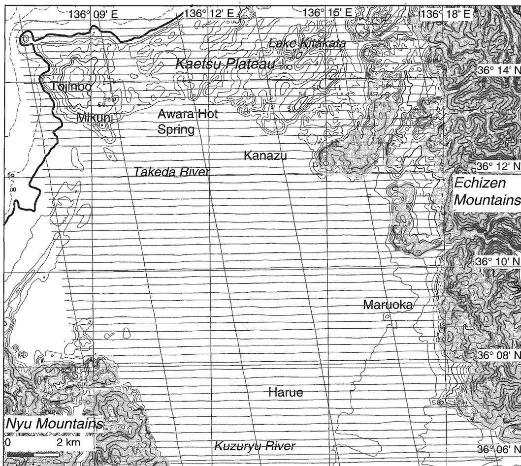
Fig. 8 Flight lines of a high-resolution aeromagnetic survey over the Fukui plain, central Japan, superimposed on a topographic map created from the DEM data with a 50 m grid by the Geographical Survey Institute (GSI). Thin solid lines show the flight lines of the GSI survey.
