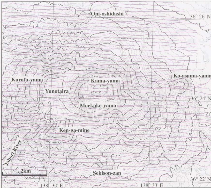
Fig. 5 Flight lines of a high-resolution aeromagnetic survey over Asama volcano, central Japan, superimposed on a topographic map created from the DEM data with a 50 m grid by the Geographical Survey Institute (GSI). Thin solid lines show the flight lines of the GSI survey. The survey was flown at an altitude of 150 m.
