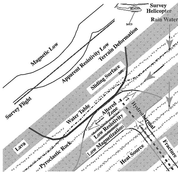
Fig. 10 Concept of the evaluation of active volcanoes' slope stability by aerogeophysical surveys.
