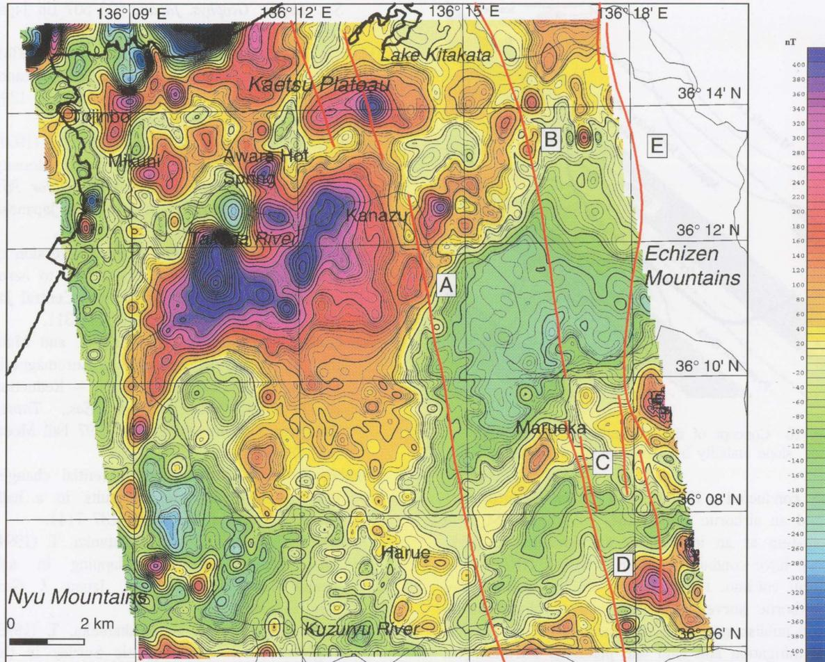
Fig. 9 Reduction to the pole anomaly map of the Fukui plain. Contour interval is 10 nT. Red solid lines indicate fault lines. The survey was flown at an altitude of 150 m, spaced 300 m apart. A: Fukui Earthquake Fault, B: Hosorogi Fault, C: Shinooka Fault, D: Fukui Eastern Earthquake Fault, E: Kengatake Fault (after the Research Group for Active Faults of Japan (1991)).
