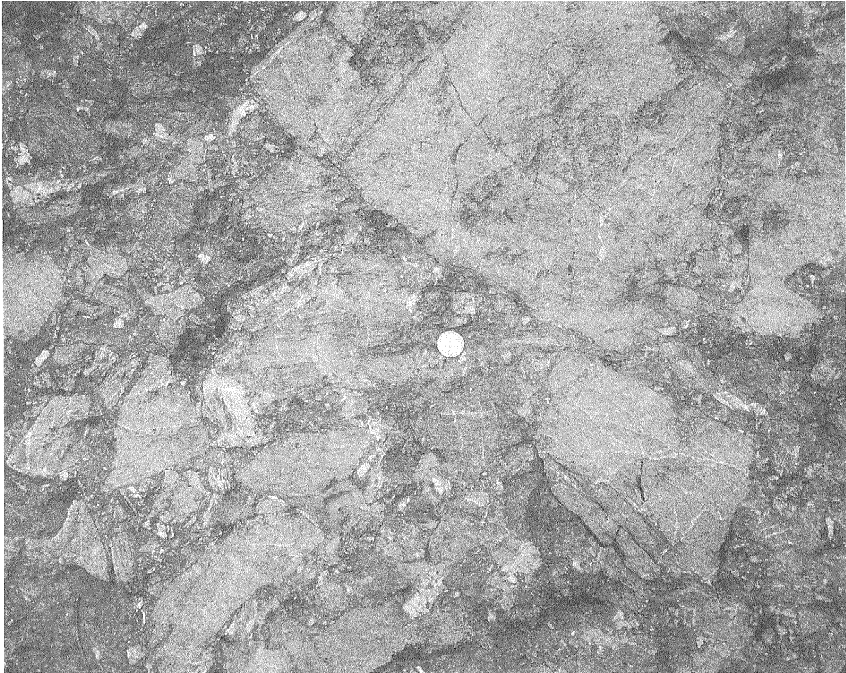
Photograph 2B Close-up of the fragments of pelitic and psammitic origin. Matrix is filled with powders of the same materials. Diameter of the coin is 23 mm.
