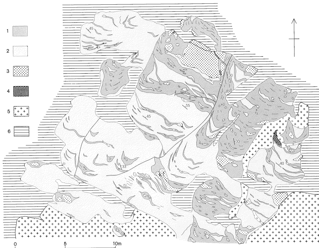
Fig. 23 Shale injection into a large siliceous shale clast in western end of the Kanayama melange, near Shimoda bridge (Lat. 35^{\circ}38'14'' , Lon. 136^{\circ}57'04'' ). 1. melange matrix (dominantly pelitic, with small clasts), 2. siliceous shale, 3. sandstone, 4. "Toishi-type" siliceous shale, 5. quartz porphyry, 6. no exposure
