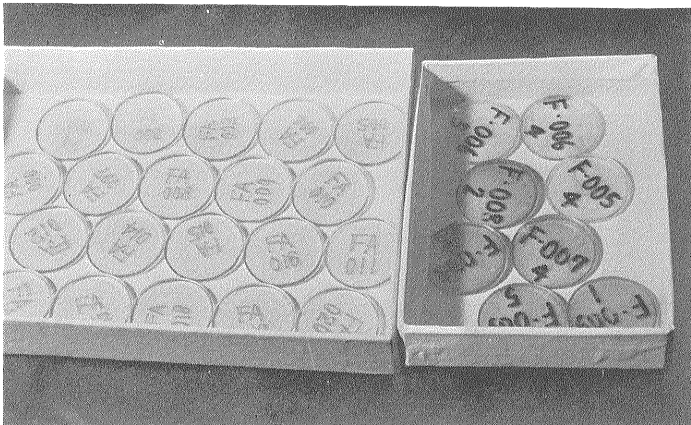
3. (Fig. 8-P) Example of glass discs (dia- meter; 31.5 mm).
