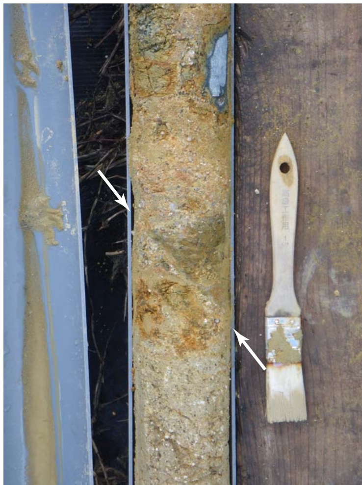
第 22 図．堀田地点 HT-4 孔コアの写真．白矢印の間が断層とみられる破断面．コア径は約 6 cm. Fig. 22. Close-up photograph of the HT-4 core in the Horita site. A shear plane is observed in between two white arrows. Diameter of the core is about 6 cm.
