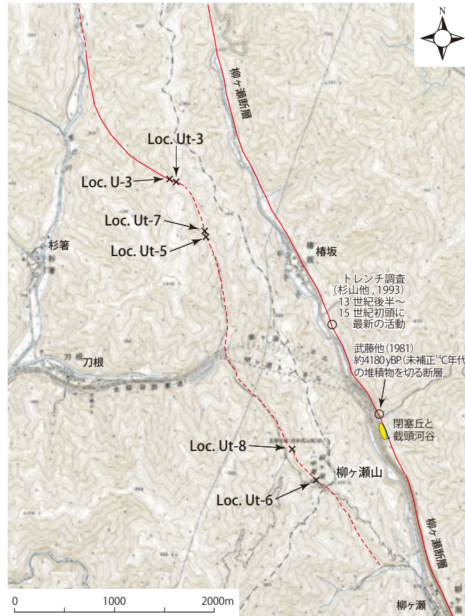
第 31 図. 柳ヶ瀬山断層及び柳ヶ瀬断層のトレースと既往調査地点. 国土地理院発行 2万 5 千分の 1 地形図「中河内」. Fig. 31. Trace of the Yanagaseyama and Yanagase faults and location of sites where precise survey has been conducted already.
